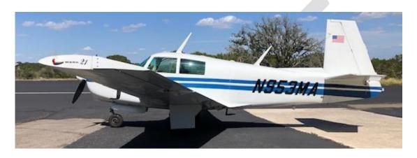
The **Mooney M20** is a family of piston-powered, four-seat, propeller-driven, general aviation aircraft, all featuring low wings and tricycle gear, manufactured by the Mooney International Corporation.
